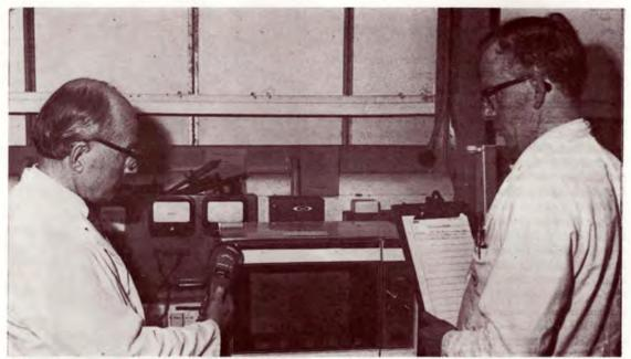
Test engineer Tom Owen, left, assisted by John Whittle, checks a microwave oven for leakage, with negative
